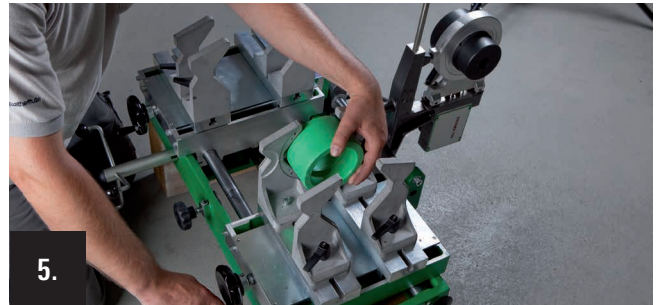
5. Hold the welding socket between the fitting clamping jaws and press it against the stops at the face side.
