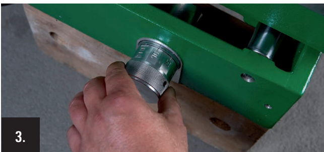
3. The welding depth of the required pipe dimension is adjusted by the turning button, which is at the left face side of the machine frame.
