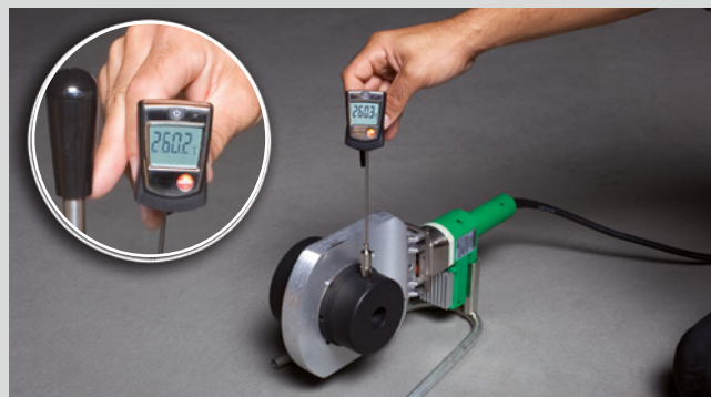
Temperature control aquatherm welding device (1400 W)
