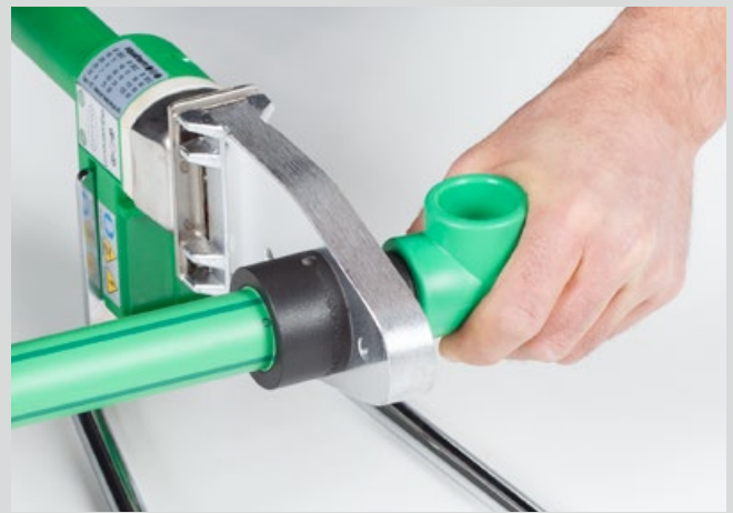
Heating-up of pipe and fitting
