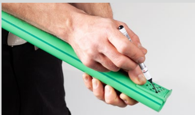
Marking of the welding depth
