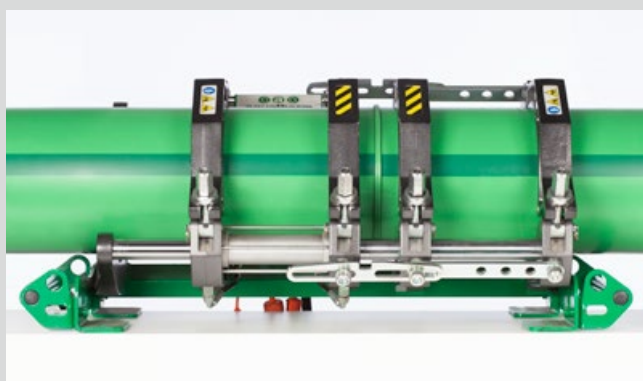
Join the pipes, cool down under pressure
