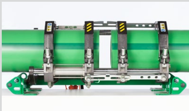
Divide the machine slide, remove heating element
