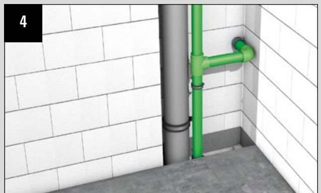
Installation of a spring leg
