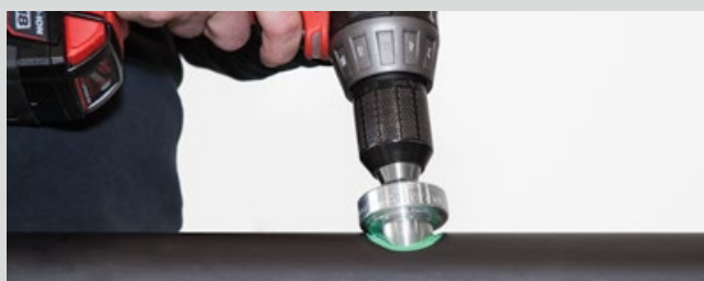
Removal of the UV layer in case of the aquatherm UV-pipe
